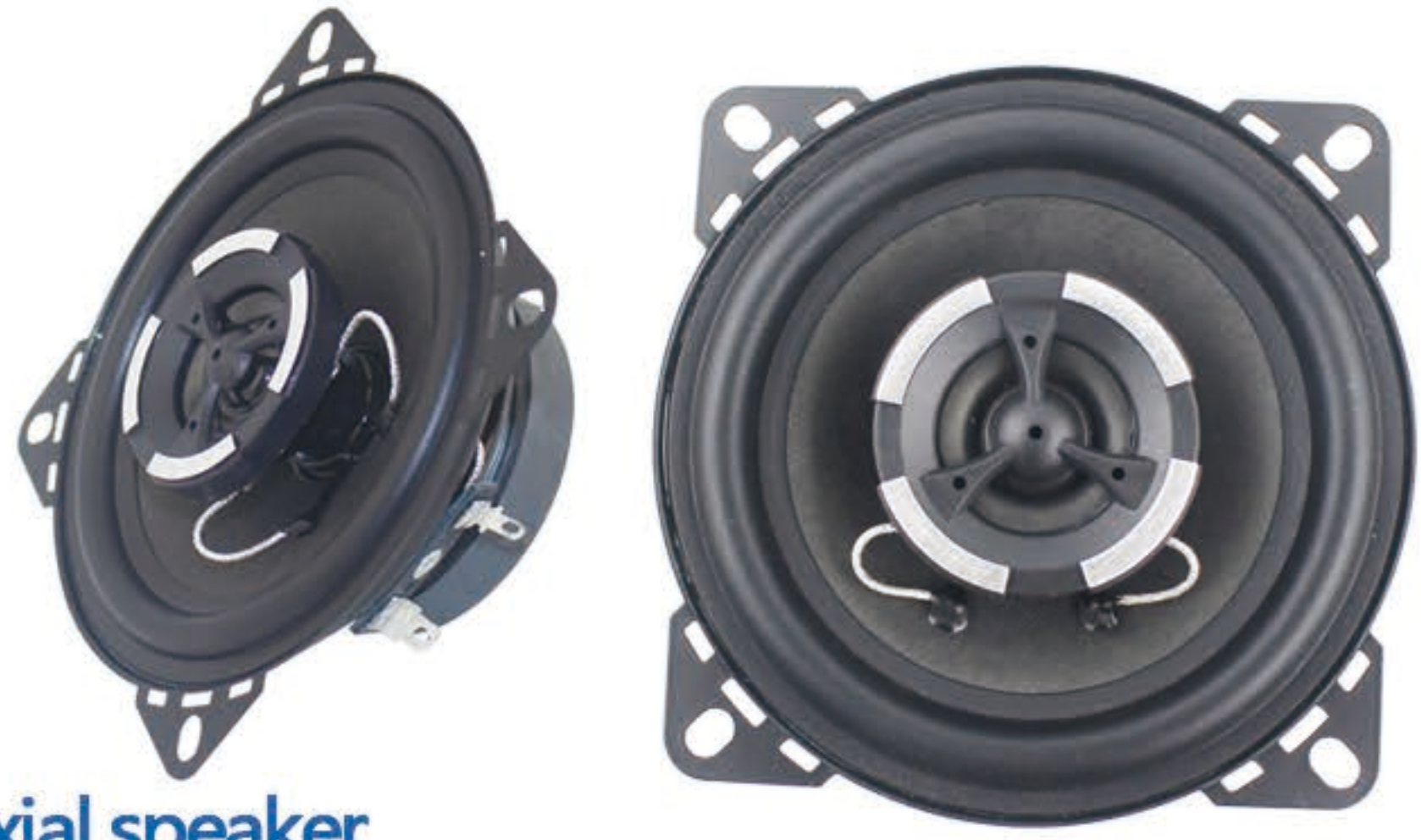
4 inch coaxial speaker Model:ZD-401 Rated power:30W Max power:100W Impedance:4Ω
